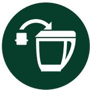
**MIND THE CUP:** Do not cover the hole in the mixing bowl lid with anything other than the measuring cup designed for and provided with your Thermomix. Do not cover the measuring cup. Otherwise, steam cannot escape, the appliance can become pressurised and may cause serious injuries.
